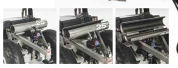
JOYSTICK CONTROLLABLE Electric Mounting Mechanism Provides Simple, Easy and Secure Attachment or Removal To Most Rigid Manual Wheelchairs With Little Or No Adjustment. Fits Widths of 15" - 20" and Rear Wheel Sizes of 24", 25" and 26"
